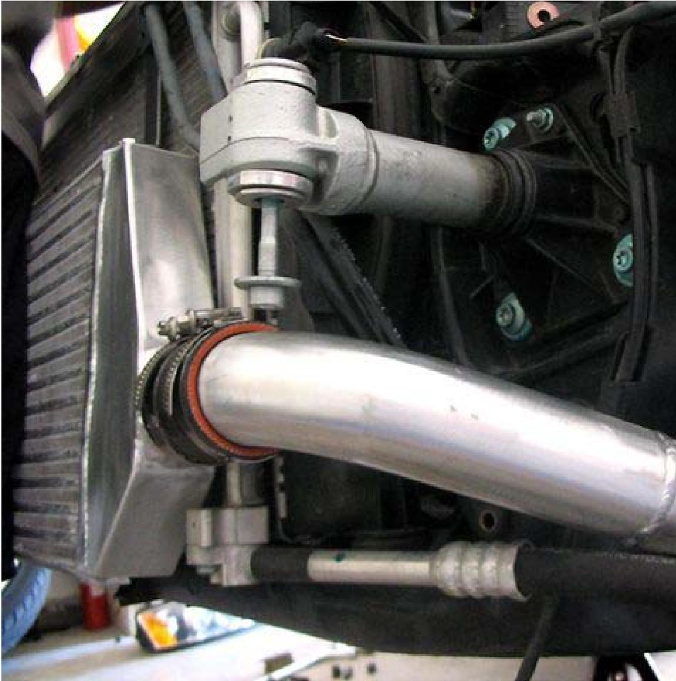
8) Double check all t-bolt clamps and intercooler alignment. Reverse install the bumper , headlamps, and belly pan.
